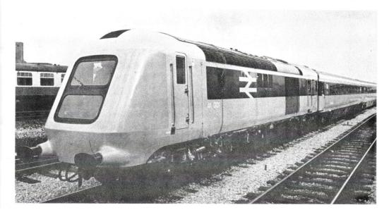
The High Speed Train, designed to be capable of 125 mph maximum speed, enables the extension and further development of the best features and principles to be found in conventional railway technology. The prototype train comprises two 56 ft. long power cars containing a 2250 hp diesel engine, at each end of seven of the 75 ft. long Mk III coaches which have been designed to set new standards of passenger comfort.
