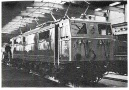
Max. T.E. 45000 lb. One Hour rating 1868 H.P. Weight 84 tons. Wheel Arrangement - Bo - Bo. Max. Speed 65 m.p.h. Built at B.R.Gorton Works. Electrical equipment by Metro-Vickers.
