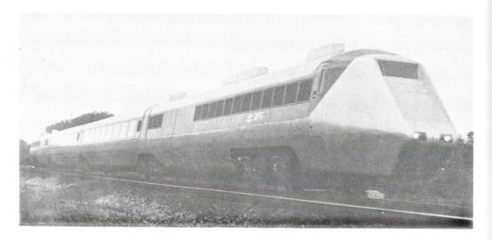
The Advanced Passenger Train projects' objectives are to reduce journey times to a minimum by exploiting fully the potential of existing track and signalling equipment and provide superlative comfort at the 155 mph top speed.
